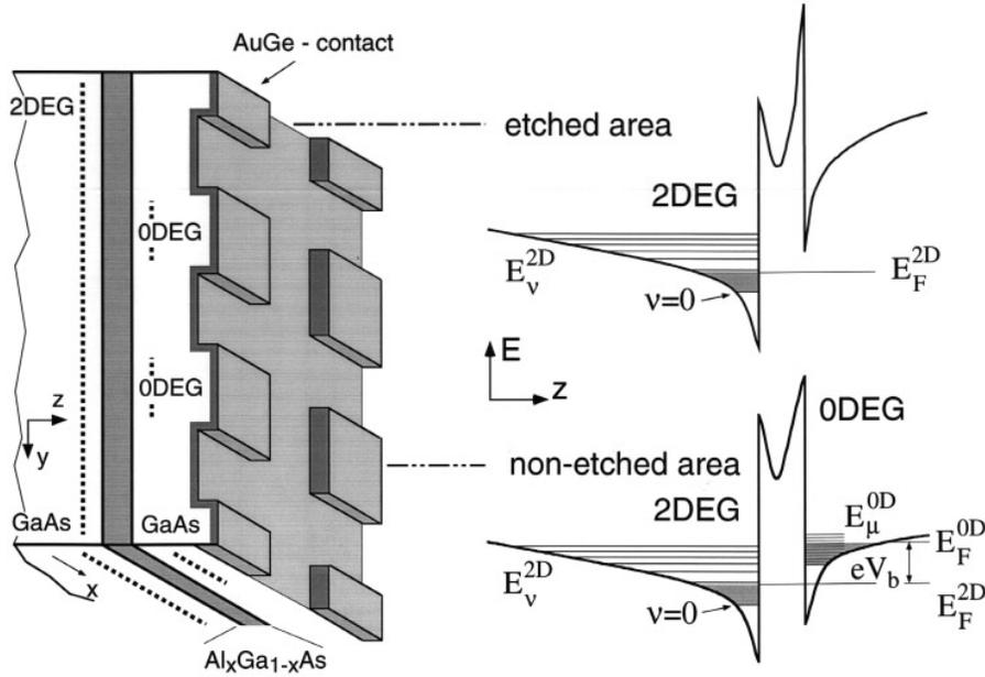
**Figure 8.** A schematic view of a 0D–2D sample is shown on the left-hand side. The corresponding conduction band profile for the etched and unetched areas of the sample is shown on the right.
