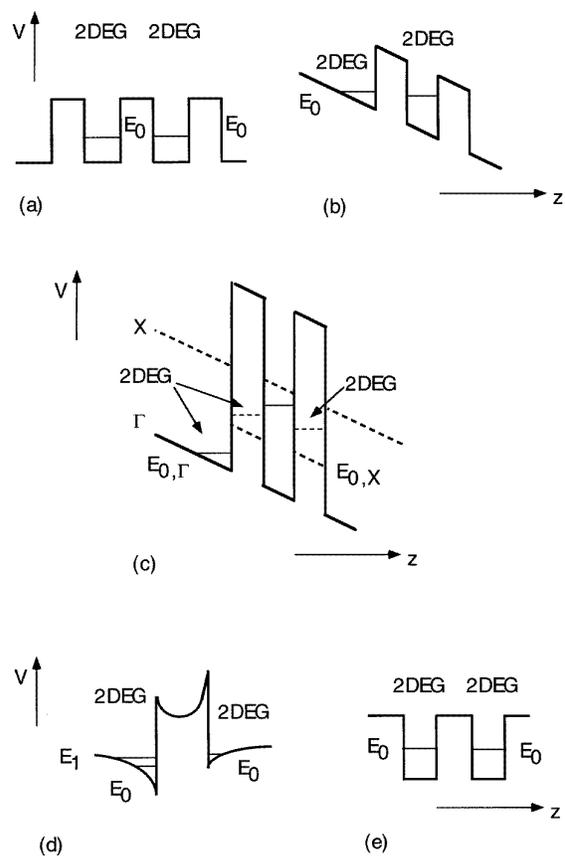
**Figure 1.** Conduction band profiles of typical 2D–2D tunnelling structures: (a) triple-barrier diodes, (b) double-barrier diode with 2D emitter, (c) double-barrier diode under hydrostatic pressure ( $\Gamma$ ,  $X$  denote the  $\Gamma$  and  $X$  conduction band profiles), (d) double heterostructure, (e) double quantum well.  $E_0$  denotes the lowest subband in each structure.
